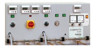
Start the machine by turning on the main switch. Each heating element is equipped with a separate switch. If the adjusted temperature is reached, the green signal of the switch disappears.
