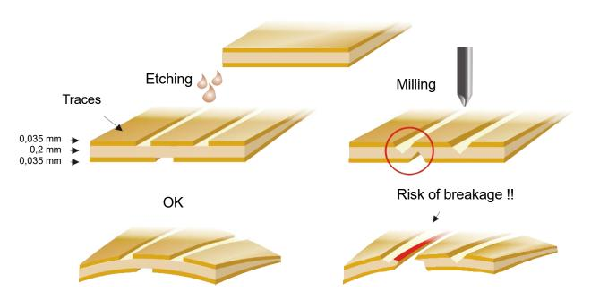
Problem: when milling, insulation channels must not lie on top of each other. Otherwise there is an extreme risk of breakage (V-scoring).
