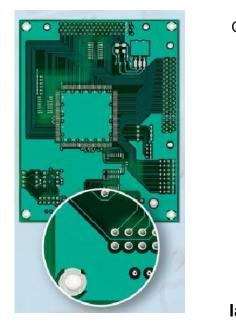
positiv presensitized boards CNC-drilling and contour routing (BUNGARD CCD/2) ┹ vacuum exposure (HELLAS LED) dip developing + rinsing + sprayetching + chemical tinning + drying (all in SPLASH CENTER) mechanical PTH (FAVORIT) lamination of solder mask (RLM 419p)
