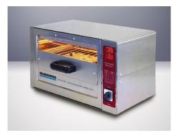
Max. substrate size: Max. placement area: Max. thickness of pcb: Height below pcb:: Components: Max. Component height: Preheating temperature: Reflow timet: Reflow temperature: 300 mm x 370 mm 245 mm x 350 mm 0,5 mm bis ~ 4 mm min. 39 mm, max. 50 mm Chip 0201 bis QFP 0,65 mm Pitch ca. 16 mm 60-260°C 0-999 Sekunden 90-300°C
