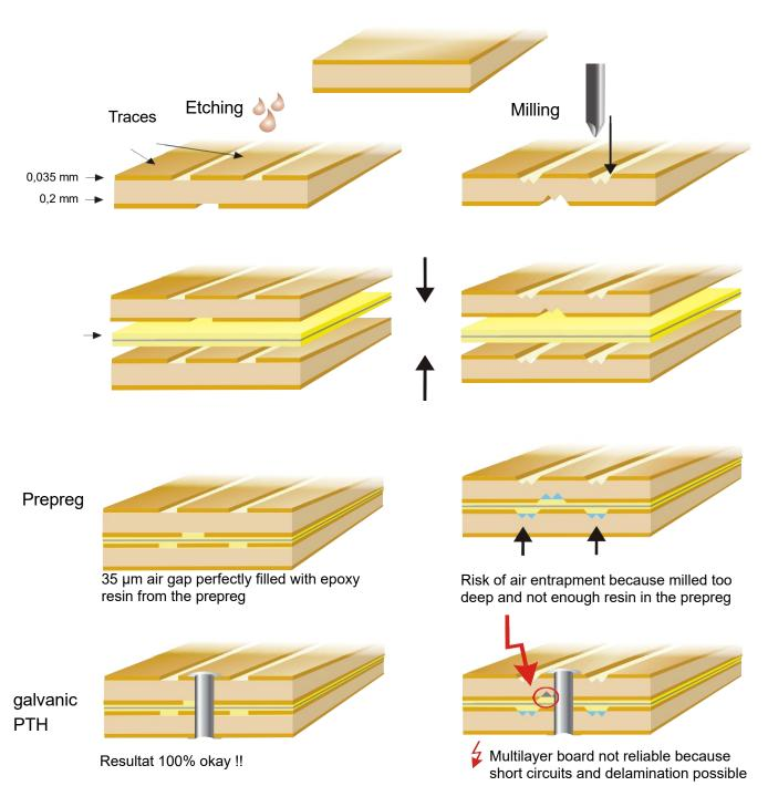
The problem with milling is that prepregs are produced worldwide only for normal copper thicknesses. They can therefore fill 35µm copper height well, but not deep insulation channels under certain circumstances. There is a considerable manufacturing risk here, because cavities can be enclosed that lead to short circuits when drilled through. If air pockets remain, there is a risk of delamination, for example during reflow soldering, due to the air bubbles expanding under heat.
