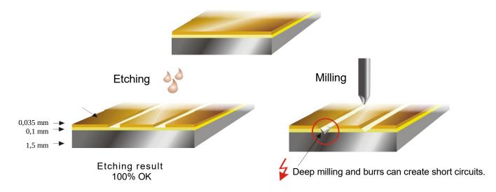
Milling problem: Too deep milling and burr formation during milling can lead to short circuits. Uncritical for etching. There, only the back and edges must be covered so as not to etch there.
