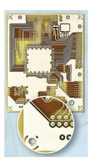
$\mathbf{J}$ CNC-drilling and contour routing (BUNGARD CCD/2)  $\mathbf{J}$ vacuum exposure (HELLAS LED) dip developing + rinsing + sprayetching + chemical tinning + drying (all in Splash CENTER) mechanical PTH
