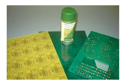
GGreen Coat is a new spray coating for all PCBs that are manually soldered.
