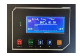
heat-phase) will be highlighted. Use the arrow keys to change the text to **HEAT**, **WELD**, **HOLD** or **COOL**. Stay on **READY** and press **SET**. The marking jumps to **TEMP** (temperature) and you can adjust the temperature between **70** and **300°C** with the arrow keys. Another press on **SET** and you can change the time between **00:01** and **08:53** (minutes: seconds).
