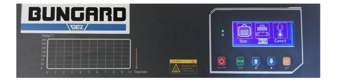
There are 5 buttons on the front panel of the unit: **POWER**, **UP**, **DOWN**, **SET**, and **RUN**, with the RUN and SET buttons being multifunction buttons. Depending on the dialogue, there are various commands above the keys that are activated by pressing the keys.
