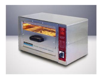
The HotAir06 SDO ONE is a solder oven suitable for lead free solder processes using SMD components.
