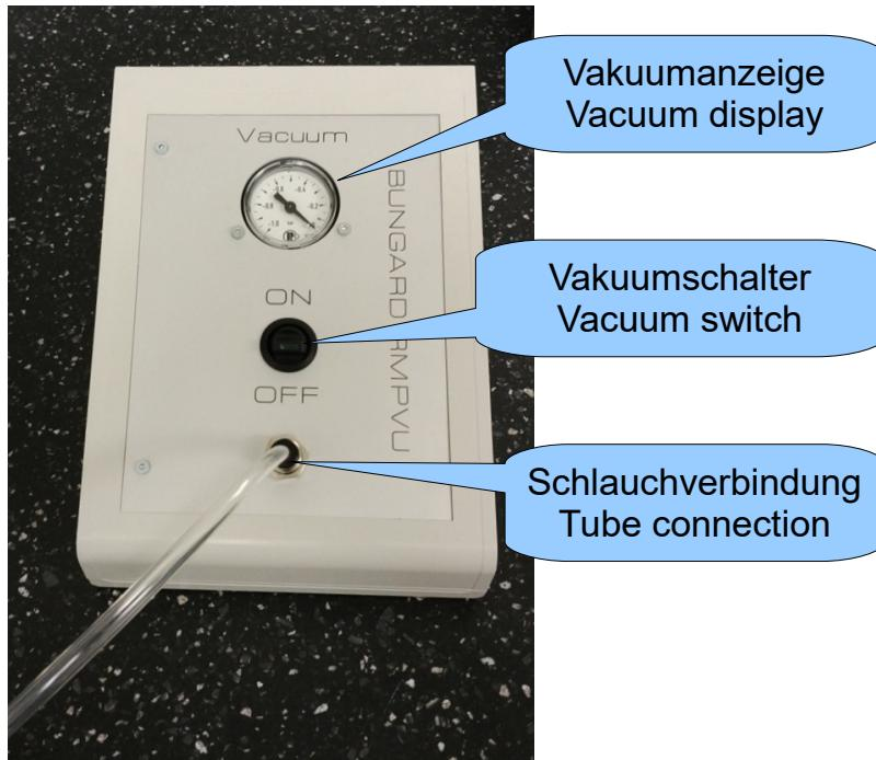
Vacuum connecting hose plugged in quick coupling /only for vacuum load !
